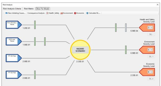
Bow-tie model is a famous risk assessment methodology. It can develop a hazard scenario in graphical and take account of the Layer of Protection analysis (LOPA) technique for detailing the consequence severity evaluation.
