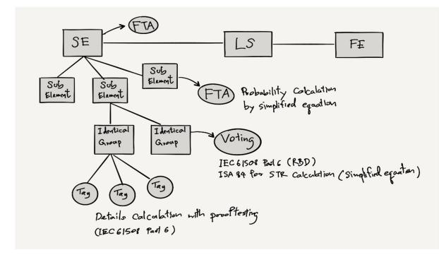
SIF design concept of InnoSIF<sup>™</sup> is more flexible to develop a complex SIF. To simplify process of design, InnoSIF<sup>™</sup> provides user-friendly interface to build a complete SIF design in one page. The subsystem configuration can be developed using Fault Tree Analysis modelling (FTA), which helps users demonstrate their design in graphical.
